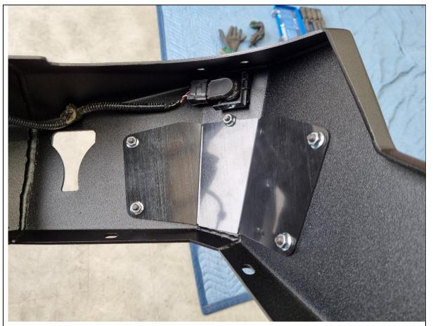
30. Fit Plastic radar cover panels to the inside of the wings of the bar, using the supplied M6 Button Head fasteners.
